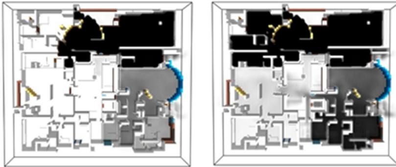
Fig. 3. Smoke spread status after 20 s and 240 s
