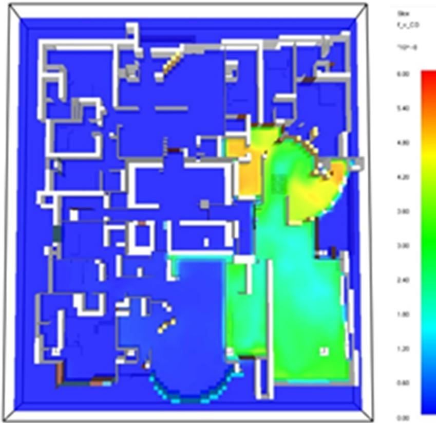
Fig. 4. CO concentration counters 50 s after beginning of fire
